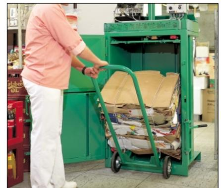
The supplied bale trolley eases baling and subsequent transport of the bale.
