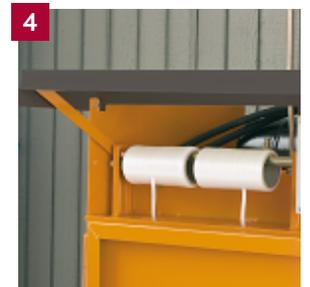
**1** Compact your waste and eject the finished bale. **2** Remove and store the bale until collection. **3** The baler has a simple control panel and is equipped with easily understood pictograms. **4** The strap rolls are easy to replace in front of the machine.
