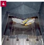
**1** The bale is tied automatically. **2** The finished bales are pushed forward. **3** The baling channel adjusts automatically to keep the bale density constant. **4** Strong and hard-wearing shear blade cuts the material.
