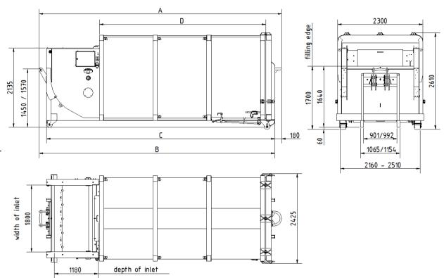
drawing shows special equipment rolls in front and hook at rear
